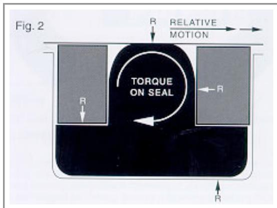
Parker T-seals have been developed to replace existing O-ring seals in long-lived hydraulic and pneumatic systems. Their ability to fit into existing grooves means that a retrofit can be made with no re-matching or major revisions to the existing hardware design. This simplifies both field changes and new equipment manufacturing.
