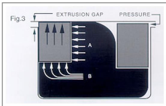
Back-up rings are on the outside diameters of piston T-seals, and the inside diameters of rod T-seals. The unique "hydraulic" loading of the back-up rings by the assembly is exposed to differential pressure causes positive back-up ring actuation. It is the positive actuation that allows the T-seal back-up rings to respond more rapidly than the
